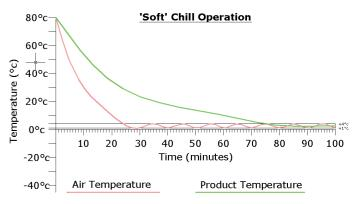
Theoretical Performance at Soft Chill Air Temp: (maintained above 0°C for protection of delicate products
