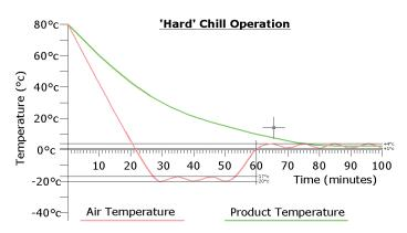
Theoretical Performance at Hard Chill Lower Air Temp. ( for more efficient cooling)
